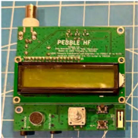
TOP TO BOTTOM: (1) PCB with pre-installed SMC parts (2) the 15 thru- hole components the builder needs to add. (3) only 2 toroids to wind (4) completed bottom of PCB (5) completed top (6) first test w. home EFHW & Emtech ZM-2 (7) Ready to go! (8) 1st QSO w. KZ9V, in US-4334 WI.
