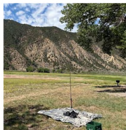
Fig 7 – Loading Coil Antenna w/Faraday cloth ground plane w/4 radials
