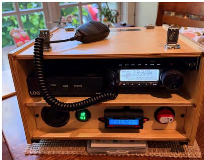
Fig. 1 - Compact HF Go-Box for POTA Activations via Air Travel
