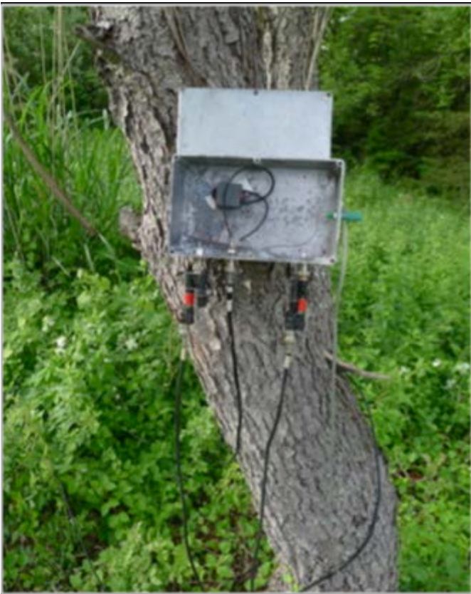
FIG. 3. The connector box is screwed to a tree, with the loop leads and signal leads hanging down. A junked die-cast EconoBox was used and minimal weatherproofing was employed. The banana-BNC connectors were temporarily used to experiment with grounding configurations.
