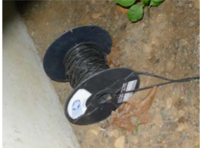
FIG. 4. The excess lead-in coax is wound onto an old empty spool, and this serves as a simple balun.
