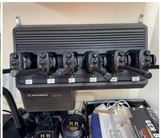
ABOVE: The CERT trailer radios. TOP LEFT: Motorola XTL1500; RIGHT: Motorola CDM1250 BOTTOM LEFT: KENWOOD 991 Dual Band; RIGHT: Rack charger for 6 Motorola HT75 HTs.
