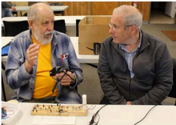
LEFT: WA1MAC explains to NZ1J about his breadboard building techniques, featuring brass tacks as contact points and stained glass copper foil tape for buses. RIGHT: WA1MAC'S DC receiver consisted of 3 distinct modules and glue stick variable inductor.
