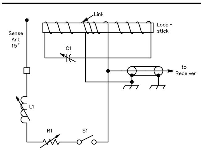
**Fig 25—Circuit of the 3.5-MHz direction finder.**
