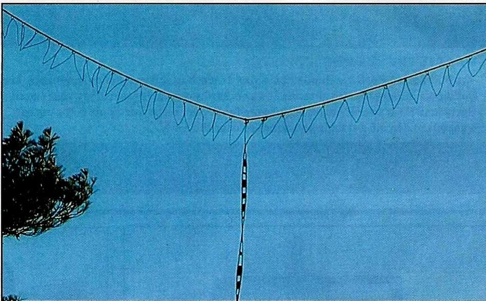
Photo A. One of the original designs constructed in 2010. It has survived multiple New England winters and is still in use at the author's QTH in Connecticut. The apexes of the wire are connected to the support rope with zip ties.
