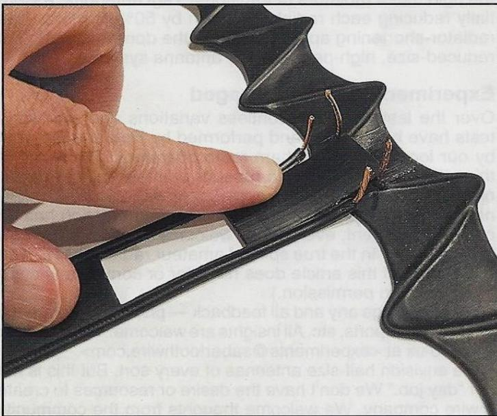
Photo D. Easy feedline attachment. Just splice in.
