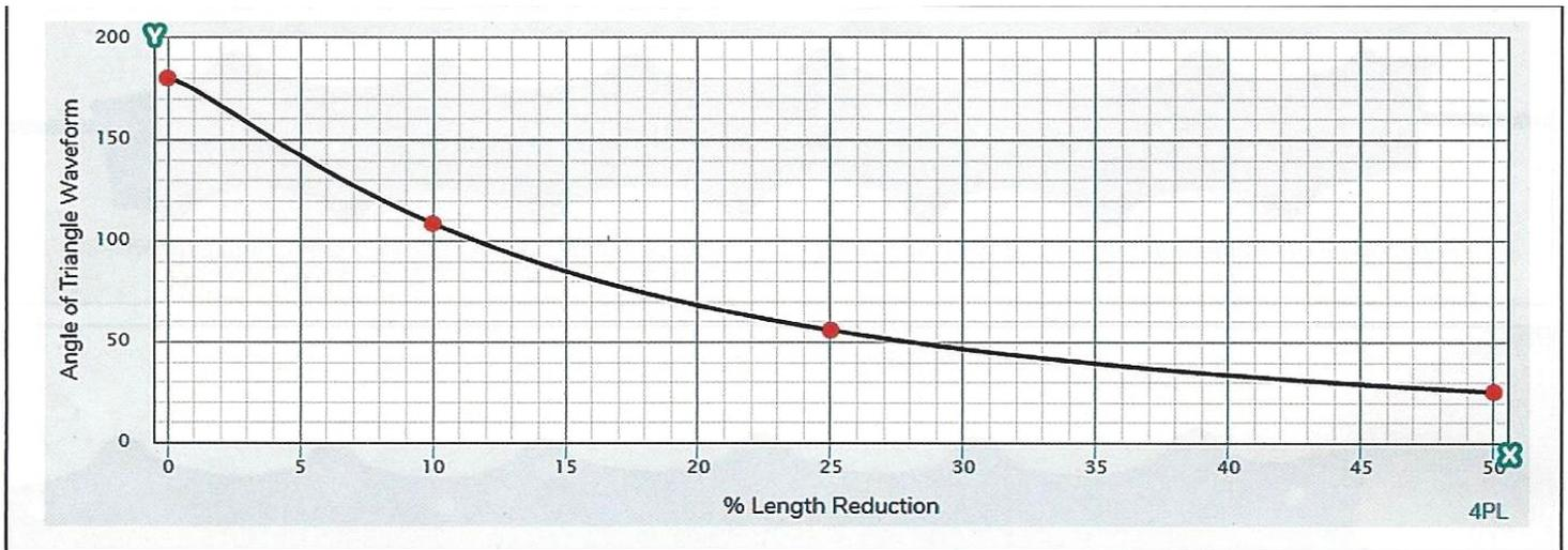
Figure 1. Plot of various data points representing antenna-wire length reduction vs. angle of waveform. (Graphic output produced by MyCurveFit.com)
