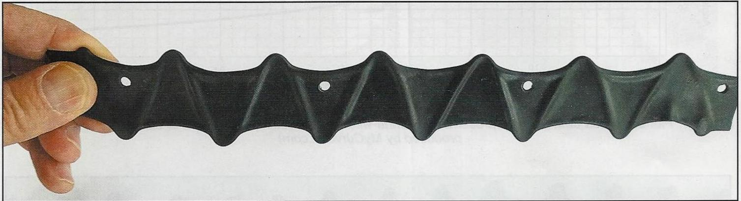
*Photo B. Examples of “Sabertooth” wire made with heat-shrink tubing. The internal wire in these examples is 16 AWG solid copper. Inexpensive 100-foot spools of 30-mm I.D. polyolefin 2:1 heat shrink tubing can be found at various online suppliers.*
