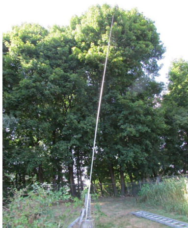
40 METER TUNED VERTICAL WITH 15 TUNED RADIALS, LOADS UP ON 40-10 WITH TUNER--KILLER ANTENNA!
