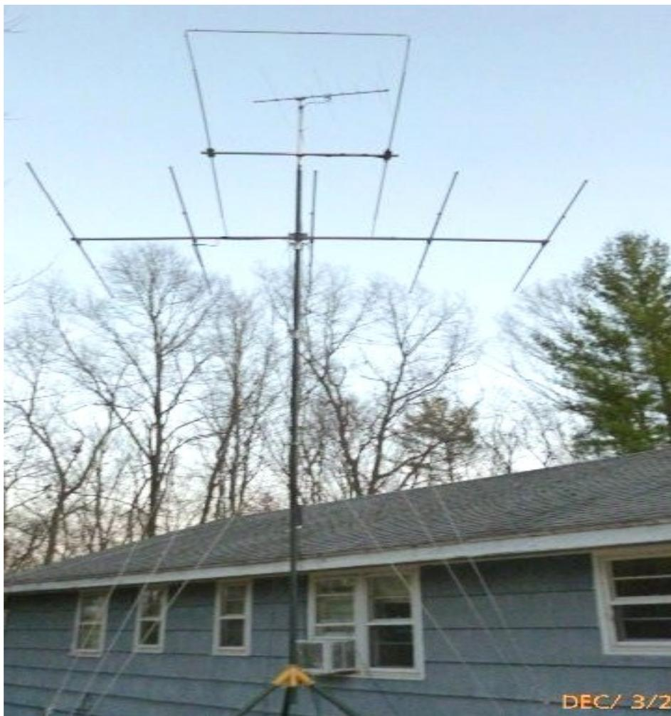
**( 5 ) Tripod w/ 5 element 6m Yagi, 10m Moxon, 2m/70cm yagi at 22 feet.**
