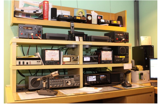
Layout from Top Row: assorted scanners, 2nd row, power supplies and recorders for 2m and 6m rigs. 3rd row 2m and 6m rotator controls and amps, 4th row: Yaesu FT736R for 6, 2, 220, and 430, and at right John's pride and joy, a Yaesu DX3000 with 75 amp PS.
