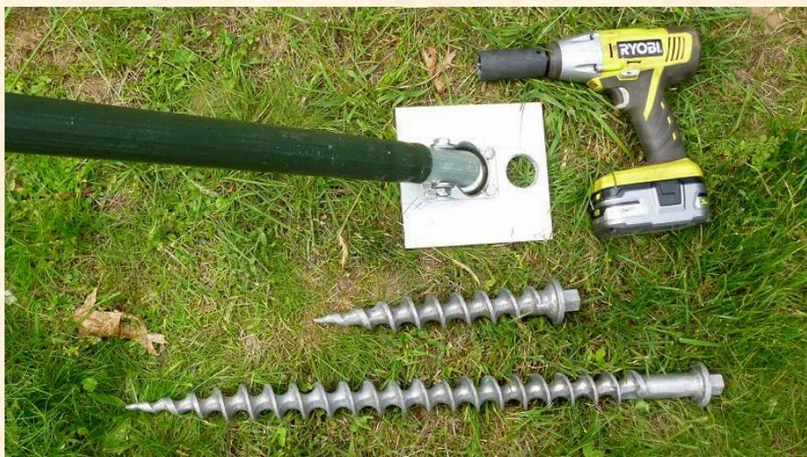
**A 1/2 Inch electric impact wrench drives the anchors easily tripods.**
