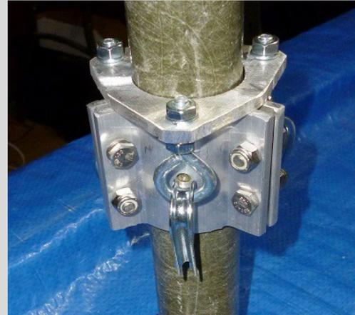
Mast joint clamp with aluminum guy ring
