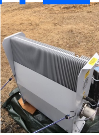
FROM K1LYP.. A 10KW RF DUMMY LOAD
