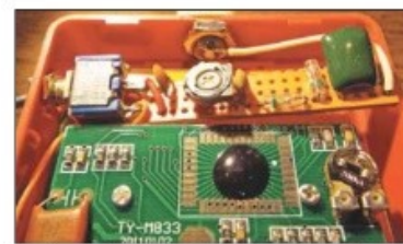
Figure 4 — The detector board mounted inside the multimeter case. The bottom of the board is insulated with plastic tape. [Richard Russo, K8GVZL, photo]
