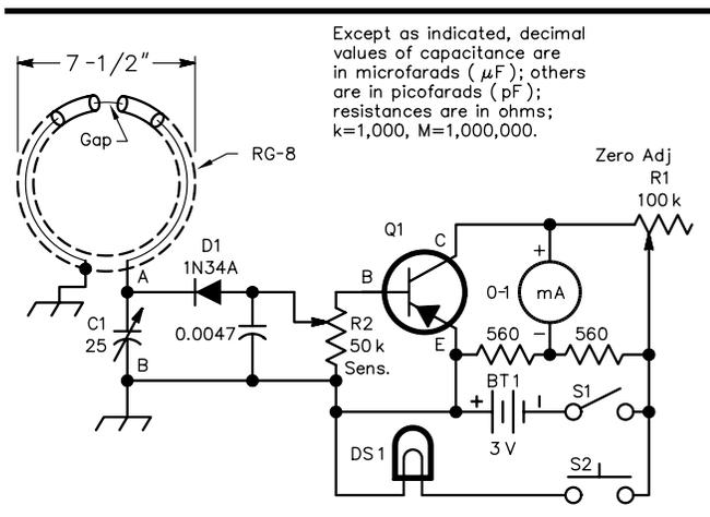
**Fig 22—The Snoop Loop circuit for 28-MHz operation.** The loop is a single turn of RG-8 inner conductor, the outer conductor being used as a shield. Note the gap in the shielding; about a 1-inch section of the outer conductor should be cut out. Refer to Fig 23 for alternative connection at points A and B for other frequencies of operation.
