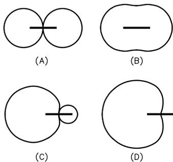
**Fig 1—Small-loop field patterns with varying amounts of antenna effect—the undesired response of the loop acting merely as a mass of metal connected to the receiver antenna terminals. The heavy lines show the plane of the loop.**
