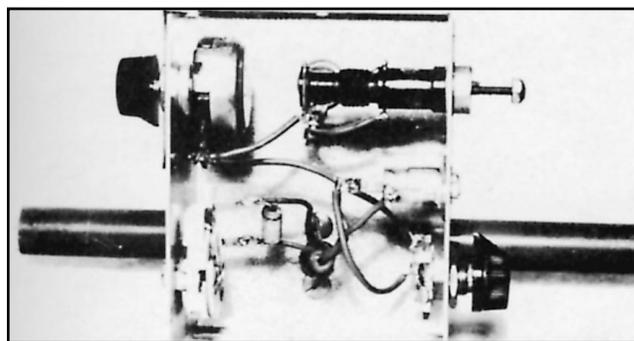
**Fig 26—Components of the 3.5-MHz RDF are mounted on the top and sides of a Channel-lock type box. In this view R1 is on the left wall at the upper left and C1 is at the lower left. L1, S1 and the output connector are on the right wall. The loopstick and whip mount on the outside.**
