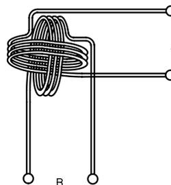
**Fig 10—An early type of goniometer that is still used today in some RDF applications. This device is a special type of RF transformer that permits a movable coil in the center (not shown here) to be rotated and determine directions even though the elements are stationary.**
