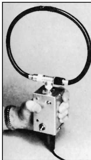
**Fig 21—The box containing the detector and amplifier is also the “handle” for the Snoop Loop. The loop is mounted with a coax T as a support, a convenience but not an essential part of the loop assembly. The loop tuning capacitor is screwdriver adjusted. The on-off switch and the meter sensitivity control may be mounted on the bottom.**
