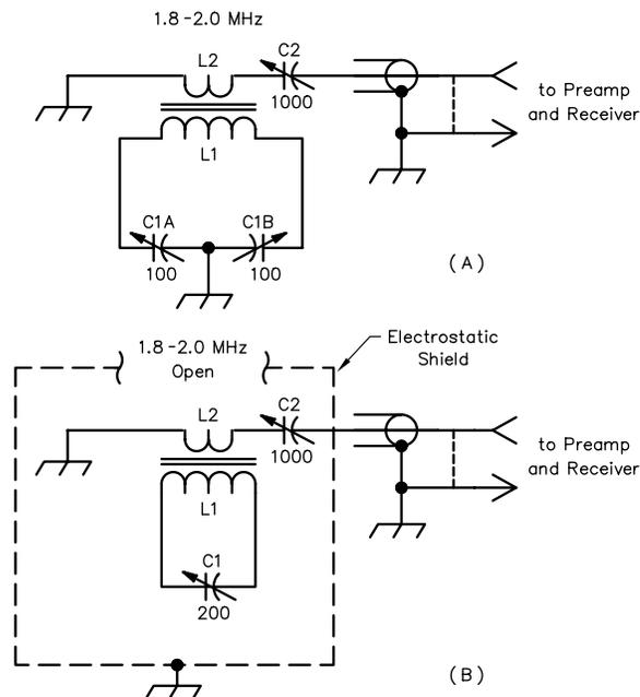
**Fig 16—At A, the diagram of a ferrite loop. C1 is a dual-section air-variable capacitor. The circuit at B shows a rod loop contained in an electrostatic shield channel (see text). A suitable low-noise preamplifier is shown in Fig 19.**
