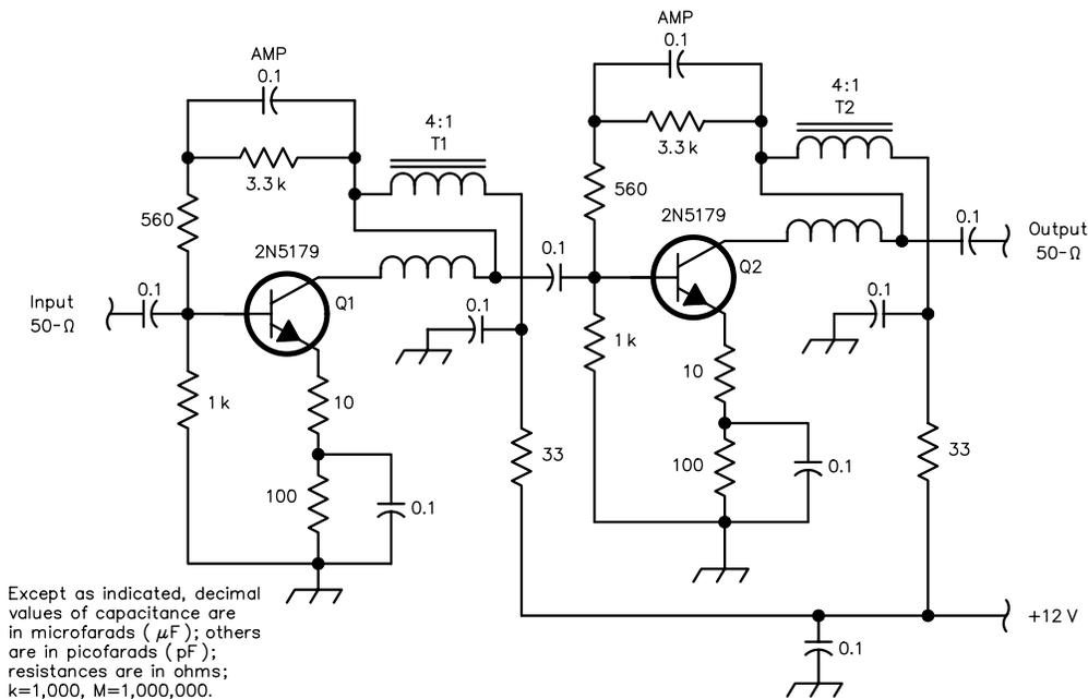
**Fig 19—Schematic diagram of a two-stage broadband amplifier patterned after a design by Wes Hayward, W7ZOI. T1 and T2 have a 4:1 impedance ratio and are wound on FT-50-61 toroid cores (Amidon) which have a  $\mu_i$  of 125. They contain 12 turns of #24 enam wire, bifilar wound. The capacitors are disc ceramic. This amplifier should be built on double-sided circuit board for best stability.**
