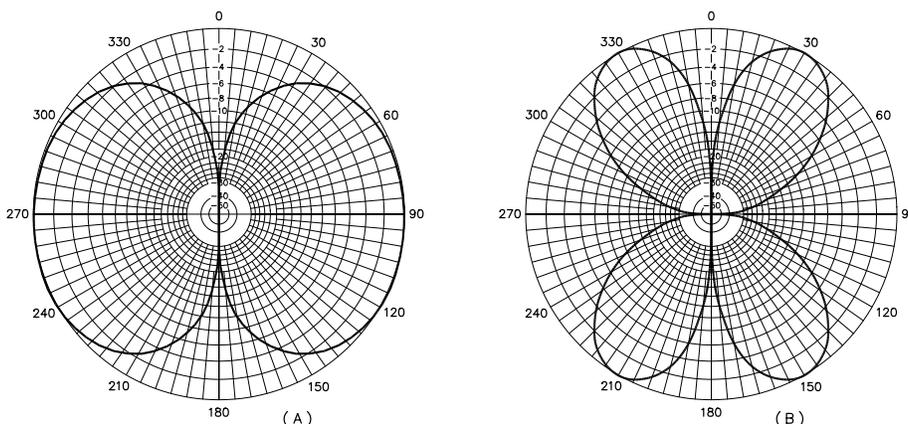
Fig 9—At A, the pattern of the Adcock array with an element spacing of  $1/2$  wavelength. In these plots the elements are aligned with the horizontal axis. As the element spacing is increased beyond  $3/4$  wavelength, additional nulls develop off the ends of the array, and at a spacing of 1 wavelength the pattern at B exists. This pattern is unsuitable for RDF work.
