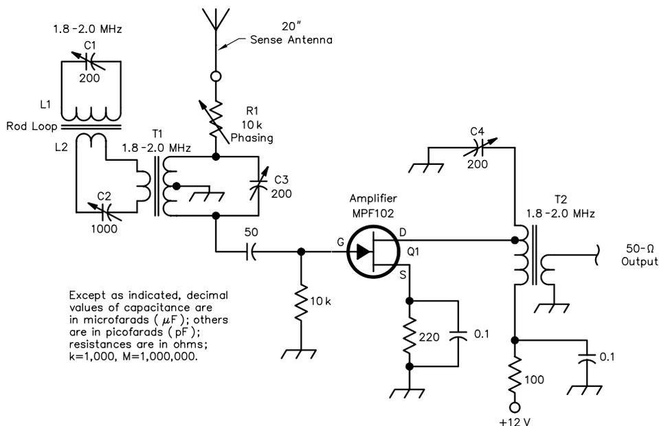
**Fig 18**—Schematic diagram of a rod-loop antenna with a cardioid response. The sensing antenna, phasing network and a preamplifier are shown also. The secondary of T1 and the primary of T2 are tuned to resonance at the operating frequency of the loop. T-68-2 to T-68-6 Amidon toroid cores are suitable for both transformers. Amidon also sells ferrite rods for this type of antenna.
