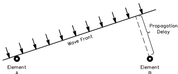
**Fig 11**—This diagram illustrates one technique used in electronic beam forming. By delaying the signal from element A by an amount equal to the propagation delay, the two signals may be summed precisely in phase, even though the signal is not in the broadside direction. Because this time delay is identical for all frequencies, the system is not frequency sensitive.
