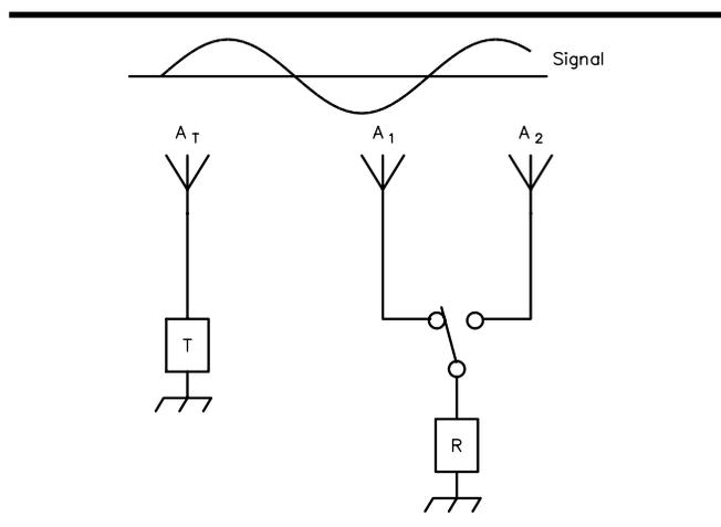
**Fig 30**—At the left,  $A_T$  represents the antenna of the hidden transmitter, T. At the right, rapid switching between antennas  $A_1$  and  $A_2$  at the receiver samples the phase at each antenna, creating a pseudo-Doppler effect. An FM detector detects this as phase modulation.
