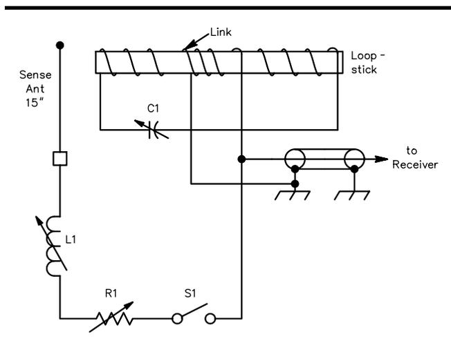
**Fig 25—Circuit of the 3.5-MHz direction finder.**
