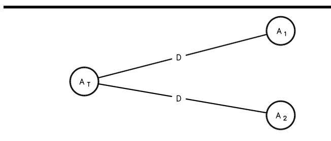
**Fig 31**—If both receiving antennas are an equal distance (D) from the transmitting antenna, there will be no difference in the phase angles of the signals in the receiving antennas. Therefore, the detector will not detect any phase modulation, and the audio tone will disappear from the output of the detector.
