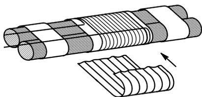
**Fig 4**—A ferrite-rod or loopstick antenna. Turns of wire may be wound on a single rod, or to increase the output from the loop, the core may be two rods taped together, as shown here. The type of core material must be selected for the intended frequency range of the loop. To avoid bulky windings, fine wire such as #28 or #30 is often used, with larger wire for the leads.
