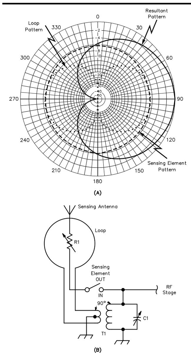
**Fig 6**—At A, the directivity pattern of a loop antenna with sensing element. At B is a circuit for combining the signals from the two elements. C1 is adjusted for resonance with T1 at the operating frequency.
