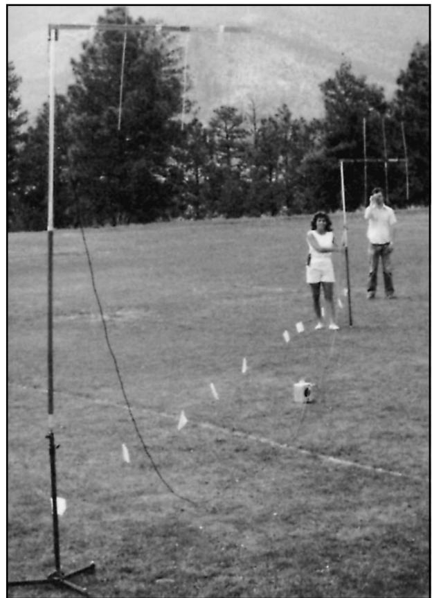
**Fig 39—Typical field setup of an interferometer. One antenna is mounted on a stand while the second is moved to find the null locations. A compass bearing is taken down the line of nulls that is marked with surveyor's flags.**
