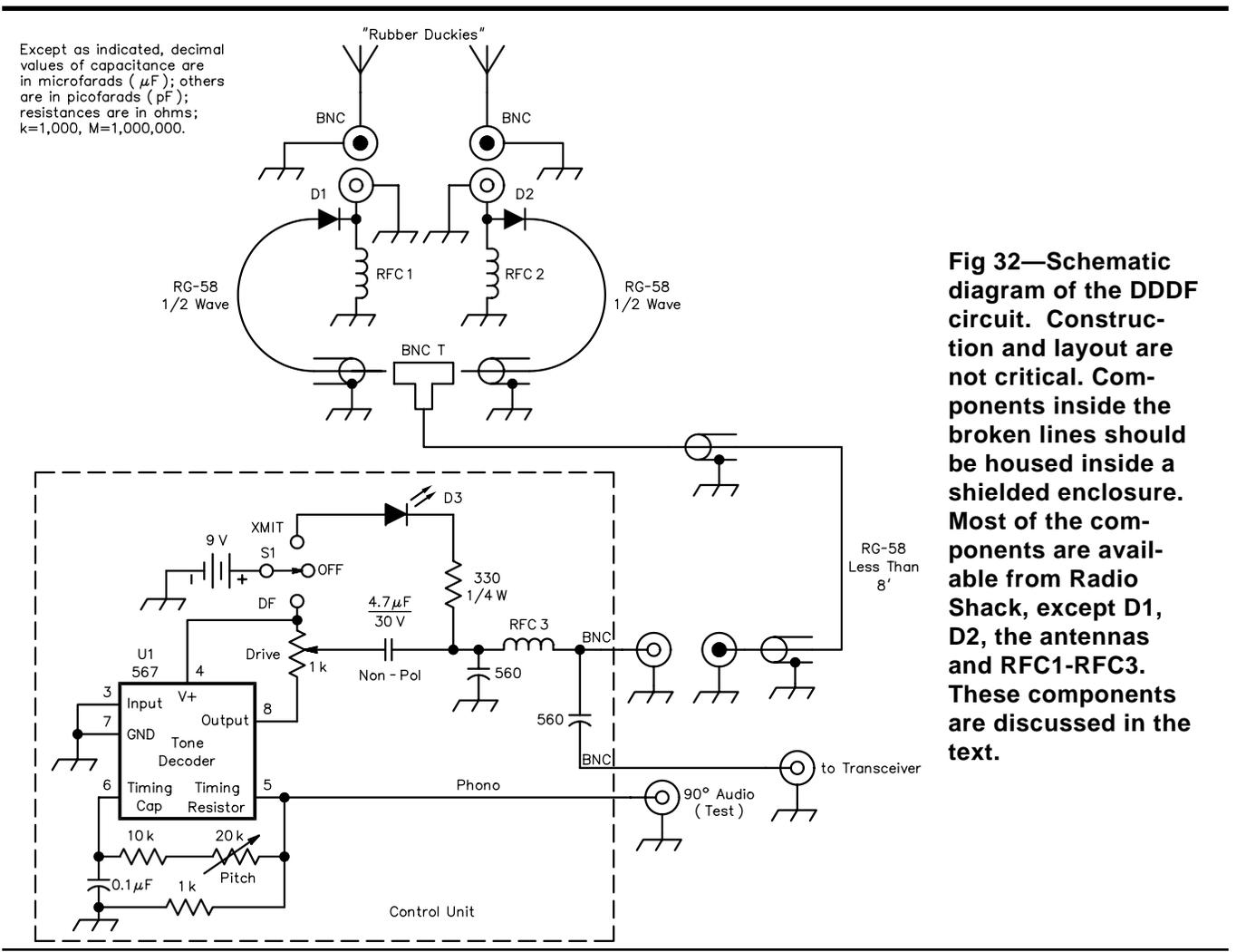
**Fig 32—Schematic diagram of the DDDF circuit. Construction and layout are not critical. Components inside the broken lines should be housed inside a shielded enclosure. Most of the components are available from Radio Shack, except D1, D2, the antennas and RFC1-RFC3. These components are discussed in the text.**
