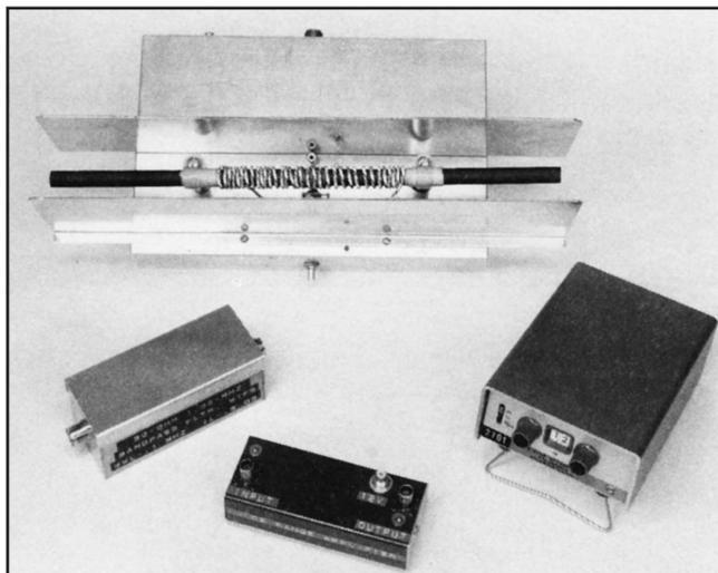
**Fig 17**—The assembly at the top of the picture is a shielded ferrite-rod loop for 160 meters. Two rods have been glued end to end (see text). The other units in the picture are a low-pass filter (lower left), broadband preamplifier (lower center) and a Tektronix step attenuator (lower right). These were part of the test setup used when the antenna was evaluated.
